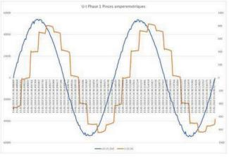
Current measurements using mu-metal current clamps
