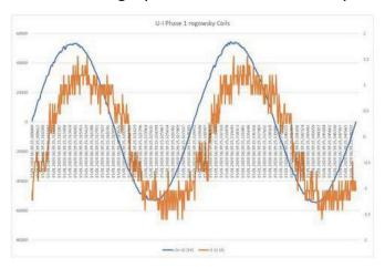
Current harmonics analysis using Ragowski Coils to measure the current
